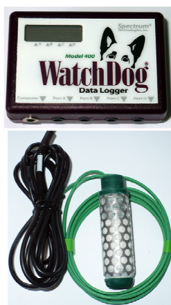
Fig. 1. 6450WD sensor (Watermark, Spectrum Technologies, Inc.) and WatchDog 400 datalogger
