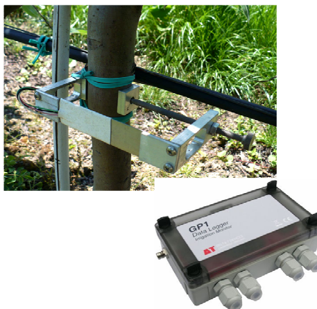
Fig. 2. DEX 100 electronic dendrometer tied with elastic bands on tree trunk and connected to the GP1 (Delta-T Devices) datalogger
